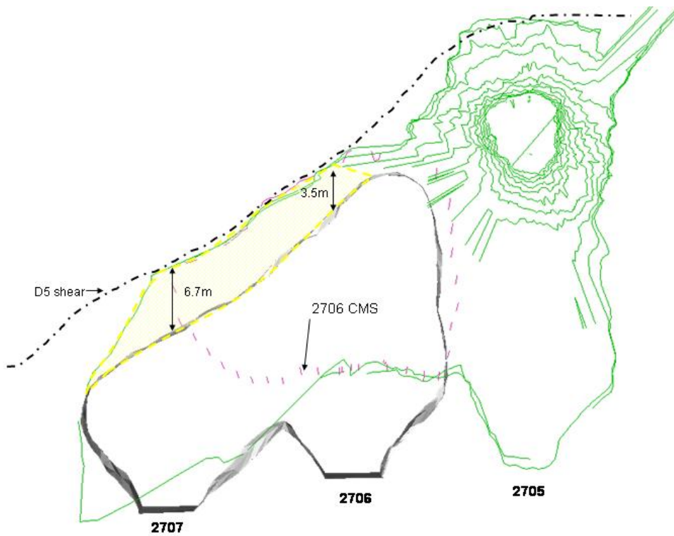
Figure 8 Cross section of the hangingwall failure above the 2707 to 2705 stopes
